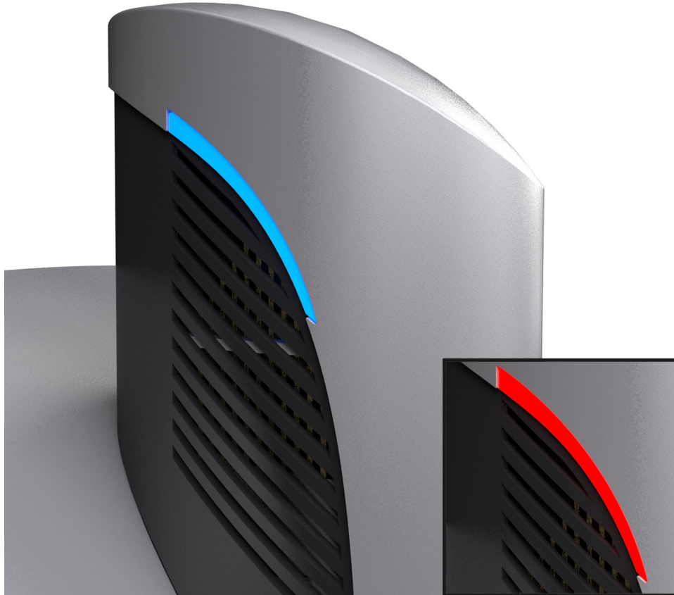
FIGURE 2.6. Status LEDs located on the side of the camera tower.
