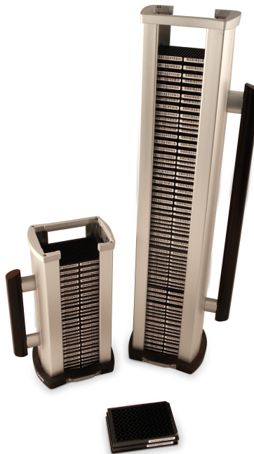
FIGURE 2.4. Fully loaded standard and high capacity stack tubes.
