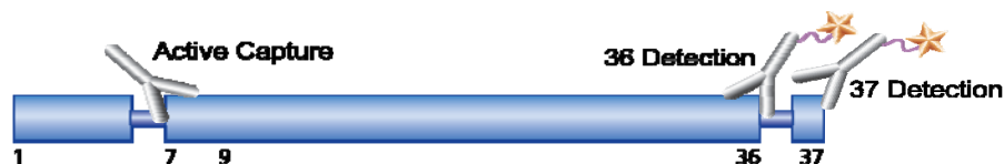
Figure 1. Sandwich immunoassay on MSD platform. The numbering convention for the different spots is maintained in the software visualization tools, on the plate packaging, and in the data files. Any spot that is not coated with a specific capture antibody is blocked with BSA to reduce non-specific binding to that spot. A unique bar code label on each plate allows complete traceability back to MSD manufacturing records.
